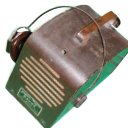
Zenith Ravox table model vacuum tube hearing aid, manufactured in 1939. The unit weighed 6 lbs. and measured 6 1/4" by 4 1/4" by 8 1/4" deep. The grill at the front conceals the microphone.
