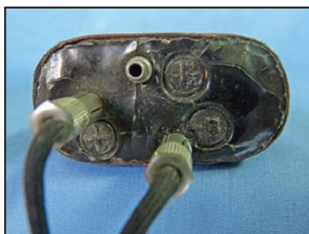
Acousticon Model 28 (Resonant Case) Carbon Hearing Aid sold in 1927 (picture on left). The Acousticon No. 2B battery (picture on right) that came with the Acousticon Model 28 Carbon Hearing Aid allowed you to select either 1 1/2 or 3 volts depending if you needed more volume for more severe hearing losses or not. It is shown here plugged into the 3 volt terminal.
