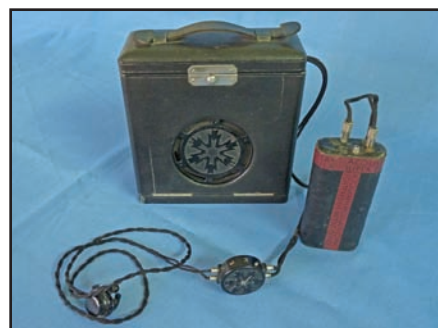
Acousticon Model 28 (Resonant Case) Carbon Hearing Aid sold in 1927 (picture on left). The Acousticon No. 2B battery (picture on right) that came with the Acousticon Model 28 Carbon Hearing Aid allowed you to select either 1 1/2 or 3 volts depending if you needed more volume for more severe hearing losses or not. It is shown here plugged into the 3 volt terminal.
