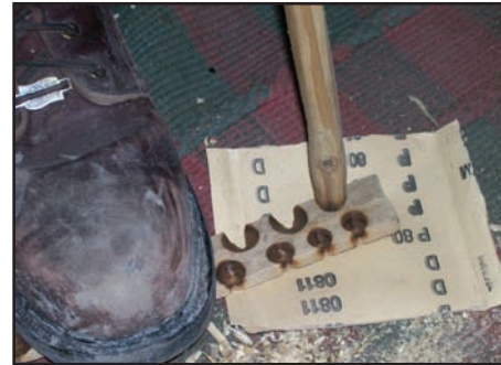
Slowly spin the spindle in the divot until the divot is large enough to keep the spindle from popping out.
