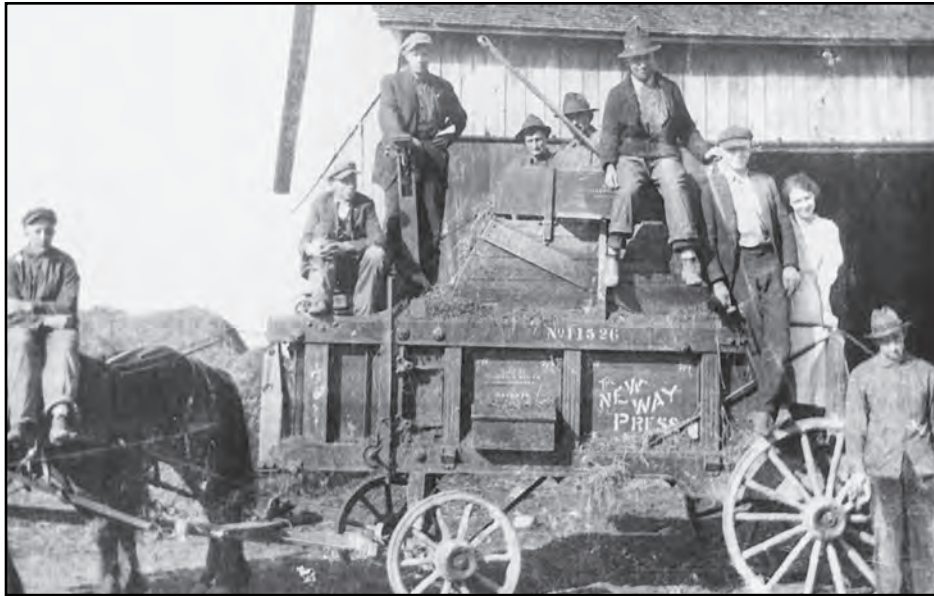
Hay was hand-fed into this hay press where it was pressed tightly while a worker installed wires or bale ties around it forming a man-made bale.
