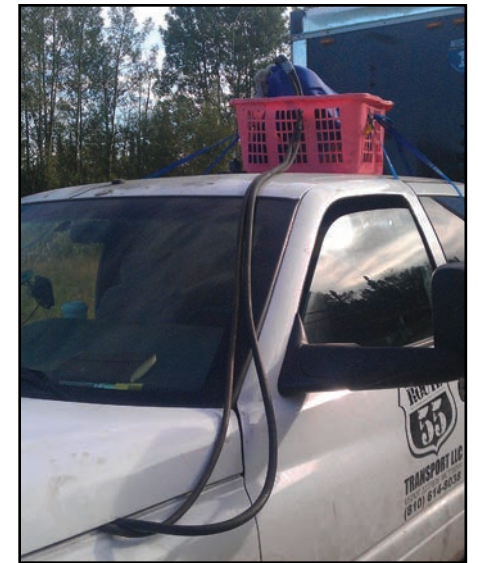
When Keith's lift pump failed, he did some unique rigging that helped him travel another 1,500 miles.
